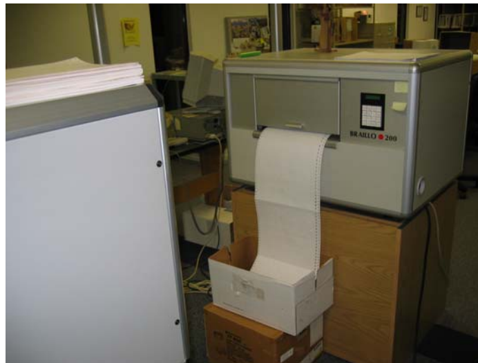
One of the computerized Braille transcribers at Seedlings.
